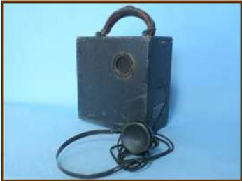
The microphone was similar to the standard carbon-shot (carbon ball) microphones used in many carbon hearing aids of the time. Note that carbon microphones had to be kept somewhat vertical.
